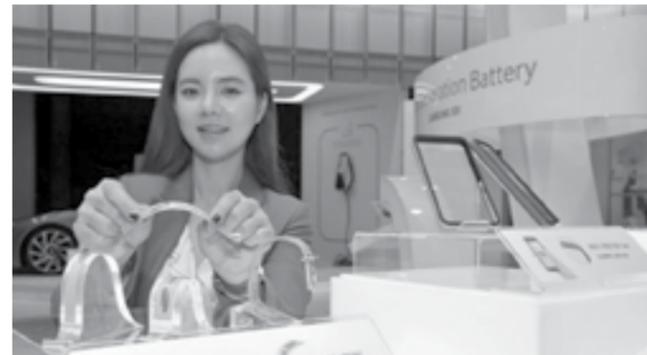
Stripe is a battery which can bend to match the contours of a person's body, such as their wrist. The flexibility is said to be akin to that of fiber, allowing it to be used in gadgets like smart bands, necklaces, t-shirt accessories and similar devices. Despite having a higher density than comparable batteries, Stripe is only 0.3mm thick.
