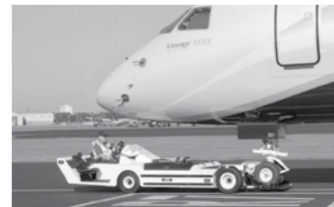
designed L16, 6V battery featuring a 4V tap to provide a true 28V ground power unit (GPU) capability for LEKTRO equipment. The 4V tap enables LEKTRO equipment to effectively service aircraft that could be otherwise harmed by potential overcharging.
